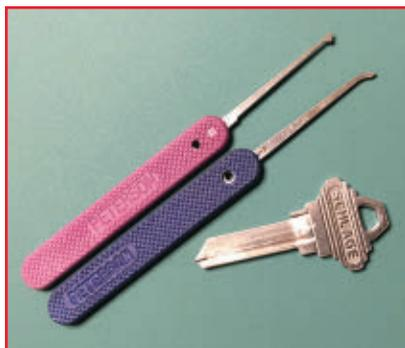
**3. Lock picks or key blanks can be used to aid in shimming.**
