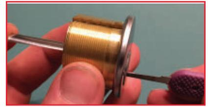
**6. If using a pick, apply light pressure to the rear of the shim and lift and lower the pin stack you're shimming.**
