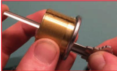
**5. While applying light pressure to the rear of the shim (the exposed end), begin moving the key and blank in and out slightly.**
